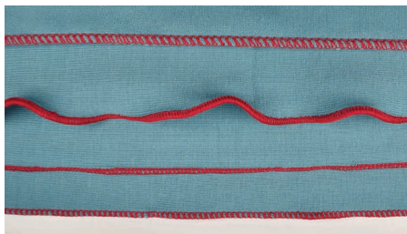
Narrow overlock/rolled hemming stitch
