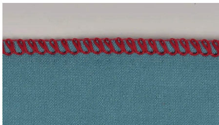
Three-thread overlock stitch - 2.8mm (7/64 inch)
