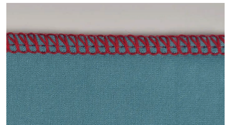
Four-thread overlock stitch
